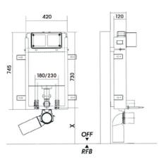
connection and corner valve 1/2", with PE wall WC bracket DN90/110, 295mm long, WC connection set, foot support, fastening material, armature group I, DIN tested, without fastening plate.
